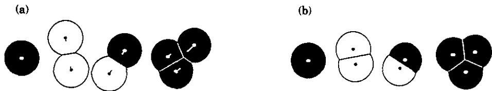
Fig. 2. Free Dirichlet domains in 2D or 3D are labeled by their "centers" (dots). Each point of one domain is closer to its center than a distance R , than to any other center. A free membrane is a spherical cap of radius R , a contact surface is the mediatrix plane between two centers. (a) At each time-step the contact lengths are calculated as a function of the center positions. The surface energy is computed, along with its spatial derivatives (Appendix A). Segments indicate the force acting on each cell, i.e. the displacement during the next time step. All cells are then moved simultaneously and a new iteration starts. (b) Equilibrium state, after \approx 1 min ( 0.055\tau_0 ). An isolated cell does not move. The competition between surface adhesion and membrane elasticity determines the final contact lengths for two and three cells. In this picture, as in Figs 5–15, dark (d) cells are more cohesive than light (l) cells, e_{dd} < e_{ll} . Here, surface energies are the same as in the cell-sorting case (Figs 10–12): e_{dM} = e_{lM} = 0 ; e_{dd} = -12E_0 ; e_{dl} = -5E_0 ; e_{ll} = -2E_0 . Corresponding surface tensions are \gamma_{dM} = 6E_0 , \gamma_{dl} = 2E_0 , \gamma_{lM} = E_0 . E_0 is a typical energy scale associated [eqn (8)] with a time scale \tau_0 of the order 10^3 sec, which is used above and in the following captions. The number of time-steps has no physical significance since we use an adaptative time discretization procedure defined in Appendix C. Cell rigidity is determined to constrain the cell size without affecting position relaxation, see Appendix B.
